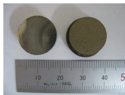
Figure 2 – (Left) SPSed CZA sample with 94% density (Right) SPSed CZA sample with 89% density
